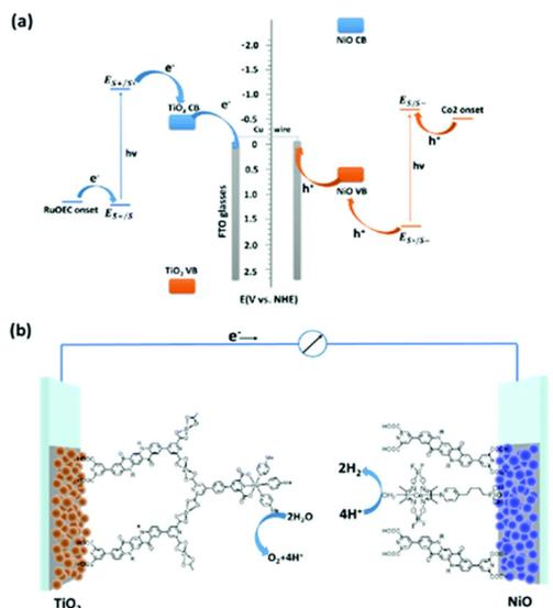
**Fig. 11** QA based photoelectrochemical cell for water splitting into hydrogen and oxygen: representation of the energy levels (a) and molecular assembly of the cell (b). Reproduced from ref. 58 with permission from the Royal Society of Chemistry, copyright 2022.
