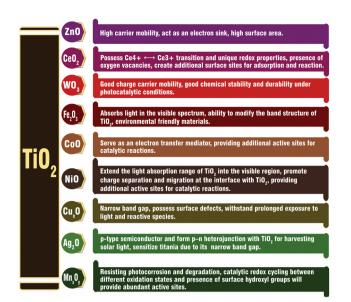
Fig. 9 Schematic representation of various metal oxides used for improving the photocatalytic hydrogen evolution activity of TiO<sub>2</sub>
