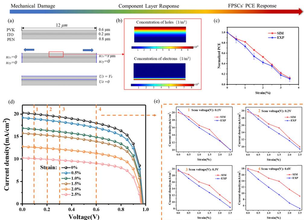
Fig. 4 (a) Two-dimensional geometric model and boundary conditions of the model; (b) the concentration distribution of electrons and holes in the perovskite layer; (c) the FPSCs' normalized PCE of experiment and simulation as a function of strain; (d) the simulated  $J$ - $V$  curves of FPSCs under tensile strains from 0% to 2.5%; (e) the terminal current density as a function of the tensile strain under the scanning voltages of 0.1 V, 0.2 V, 0.3 V and 0.6 V.
