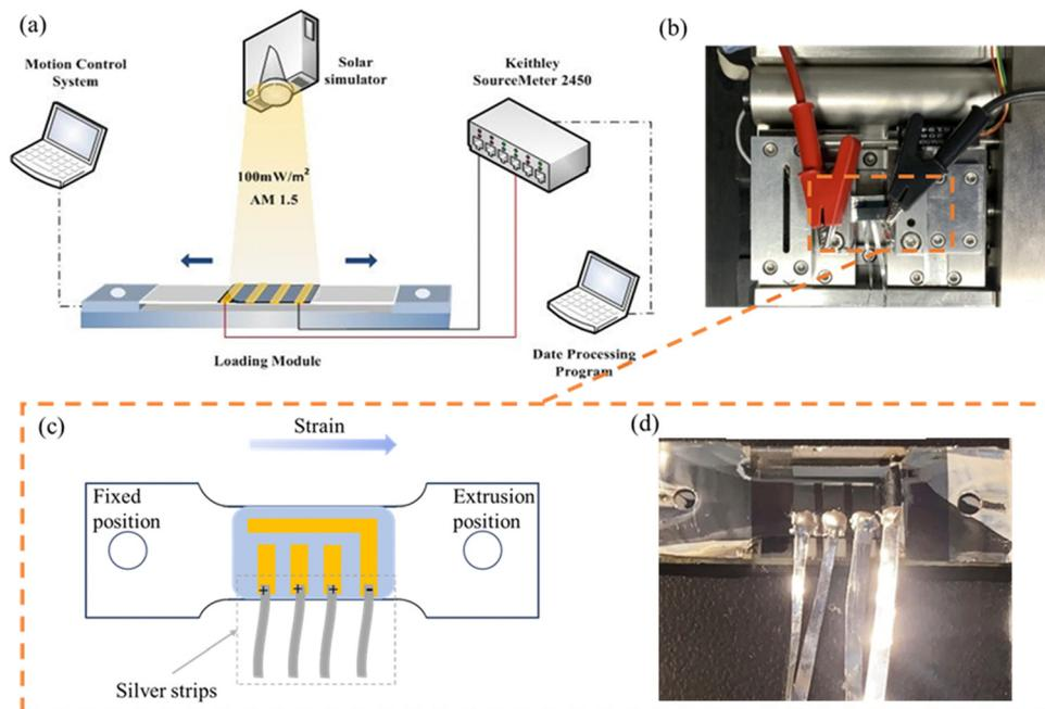
Fig. 1 Mechanical and electrical test of FPSCs. (a) Schematic diagram of the *in-situ* mechanical-photoelectrical testing platform; (b) the *in-situ* tensile test apparatus; (c) and (d) the tensile testing sample of FPSCs prepared on a dog-bone shape flexible substrate.
