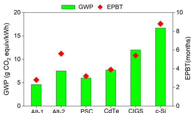
Fig. 5 Comparison of GWP and EPBT of Alt-1 and Alt-2 ld-PSC with reference PSC and other commercial PV technologies. These comparisons are made under the assumption of an average global solar irradiation of 1700 kW h m<sup>-2</sup> year<sup>-1</sup>, and a performance ratio of 0.75.
