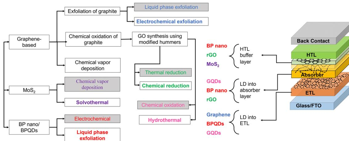
**Fig. 1** Various LD material integration into PSC structure and possible synthesis routes. The color-coded processes represent possible synthesis routes, with bold colored ones indicating the selected routes for LD materials in this study. The processes highlighted in grey color have been excluded from consideration due to their impracticality for commercial-scale production, as they are both energy and time-intensive.
