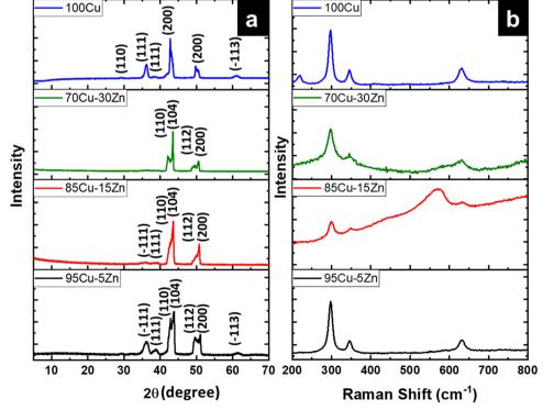
Fig. 3 (a) XRD patterns for the as-annealed 95Cu-5Zn, 85Cu-15Zn, 70Cu-30Zn, and 100Cu, (b) Raman Spectra of the 95Cu-5Zn, 85Cu-15Zn, 70Cu-30Zn, and 100Cu samples
