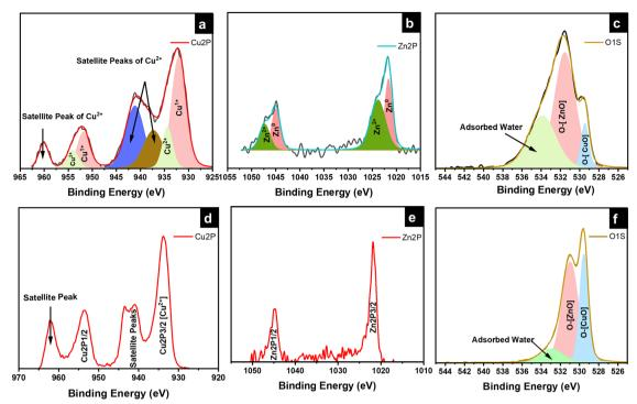
High-resolution XPS spectra of the (a)-(c) as-anodized and (d)-(f) annealed 95Cu-5Zn sample.
