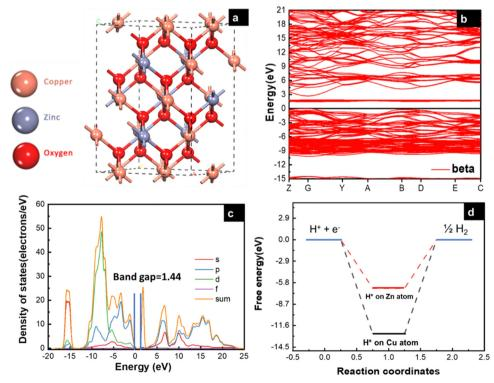
Fig. 1 (a) Side-view of CuZnO bulk (95% Cu, 5% Zn), (b) electronic band structure specified by the Fermi level with black line, (c) partial density of states (PDOS), and (d) free energy (eV) of H\* adsorption on Cu and Zn atom.
