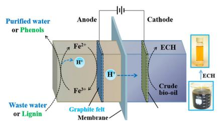
Fig. 13 Schematic illustration of low-energy ECH of bio-oil: experimental setup. Reprinted with permission from ref. 41. Copyright 2018 American Chemical Society.
