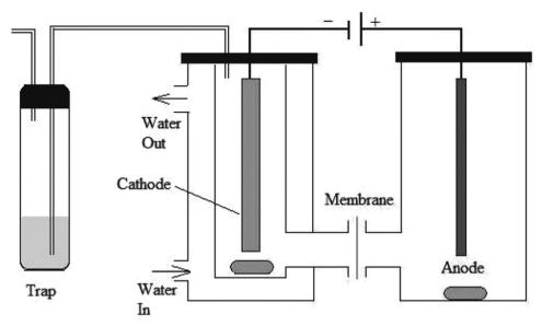
Fig. 11 Electrochemical hydrogenation cell setup for ECH of water-soluble bio-oil.<sup>72</sup>
