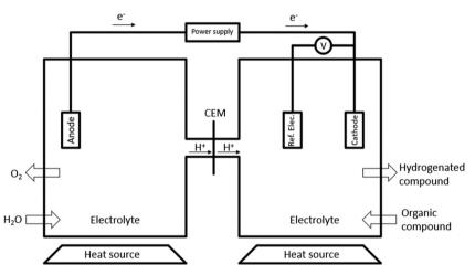
Fig. 6 A typical H-type cell, where the two chambers are separated by a membrane
