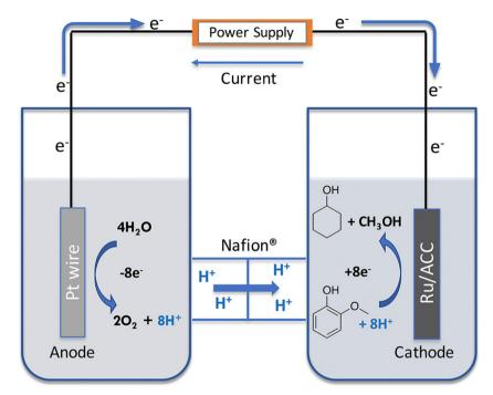
Electrocatalytic hydrogenation in a two-chambered H cell. Reprinted with permission from ref. 56. Copyright 2019 American Chemical Society.
