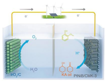
Fig. 7 Schematic of ECH of quaiacol into KA oil integrated with O2 production, equipped with PtNiB/CMK-3 and IrO2/C as the cathode and anode, respectively. Reprinted with permission from ref. 42 Copyright 2019 Wiley.
