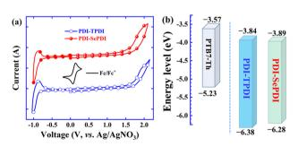
Fig. 2 CV curves of asymmetric acceptors PDI-TPDI and PDI-SePDI (a) and energy level alignment for the used donor and acceptors (b).
