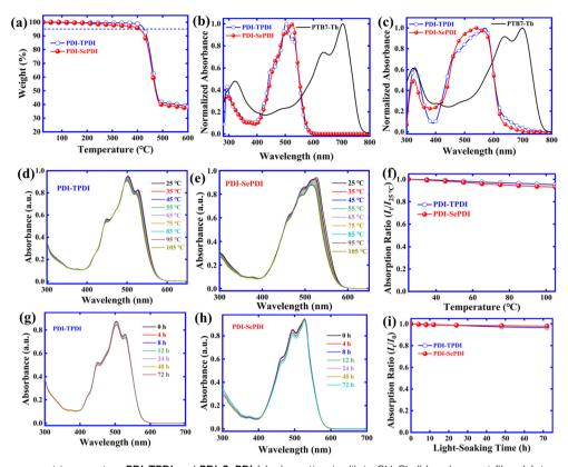
Fig. 1 TG curve for asymmetric acceptors PDI-TPDI and PDI-SePDI (a), absorption in dilute CH<sub>2</sub>Cl<sub>2</sub> (b) and as neat films (c), temperature-dependent absorption for PDI-TPDI (d) and PDI-SePDI (e) as well as the curve of maximum absorption intensity relative to temperature (f), changes for UV-vis absorption for PDI-TPDI (g) and PDI-SePDI (h) in chlorobenzene after illumination, and absorption intensity variation trend relative to lightsoaking time (i).
