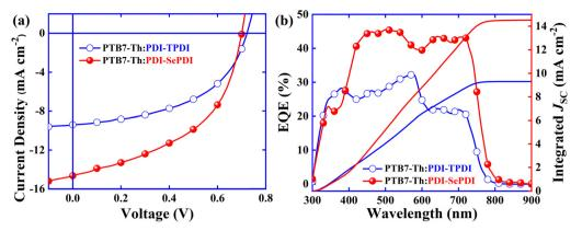
Fig. 4 Best J-V (a) and EQE (b) curves for **PDI-TPDI** and **PDI-SePDI-**based devices.
