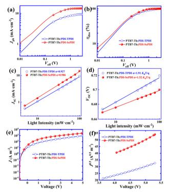
Fig. 5 Plots of  $J_{\rm ph}$  vs. effective voltage ( $V_{\rm eff}$ ) (a),  $\eta_{\rm diss}$  vs.  $V_{\rm eff}$  (b),  $J_{\rm SC}$  vs. light intensity (c),  $V_{OC}$  vs. light intensity (d), J-V curve (e) and fitting  $J^{0.5}-V$  curve (f) for PDI-TPDI and PDI-SePDI-based devices.
