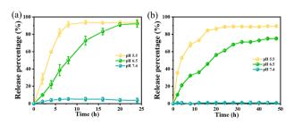
Fig. 3 TCS release from TCS@ZIF-8 nanoparticles (a) and nanofibrous
