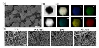
Fig. 2 (a) SEM image of TCS@ZIF-8; (b) TEM images of TCS@ZIF-8; (c) element distribution of TCS@ZIF-8; (d) SEM images of electrospun membranes
