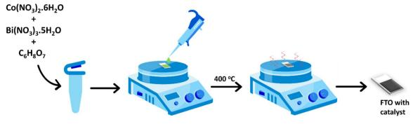
Fig. 1 Schematic of the synthesis of  $Co_aBi_bO_X$  catalysts on FTO. The procedure involves: (i) mixing Co(n) nitrate and Bi(nn) nitrate in citric acid solution, (ii) deposition of the solution onto FTO substrate, and (iii) drying and annealing the FTO-deposited metal salts.
