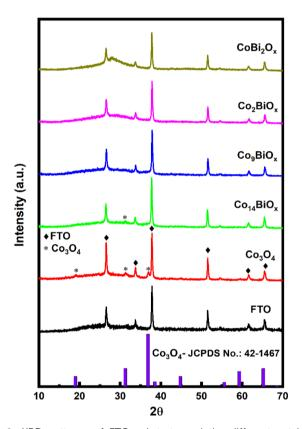
Fig. 2 XRD patterns of FTO substrate and the different catalysts synthesized in situ on FTO substrates, namely  $\text{Co}_3\text{O}_4$ ,  $\text{Co}_{14}\text{BiO}_x$ ,  $\text{Co}_2\text{BiO}_x$ , and  $\text{CoBi}_2\text{O}_x$ . The XRD pattern of  $\text{Co}_3\text{O}_4$  obtained from the JCPDS database is included for reference.
