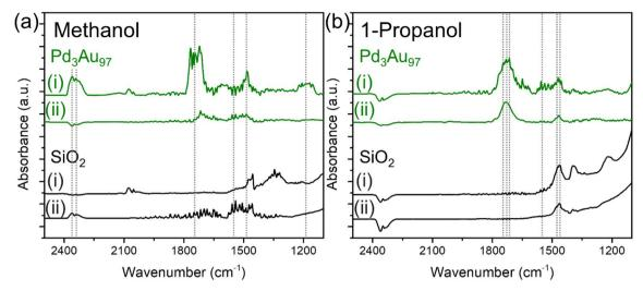
Fig. 4 In situ FTIR spectra in the  $2500-1100 \text{ cm}^{-1}$  region collected (i) during the oxidation of (a) methanol and (b) 1-propanol over Pd<sub>3</sub>Au<sub>97</sub> RCT-SiO<sub>2</sub> (green) and RCT-SiO<sub>2</sub> (black) at 423 K for 1.5 h and followed by (ii) purging in He for 2 h. Reaction conditions: 4% alcohol and 10% O<sub>2</sub>, balanced in He; total flow rate = 20 mL min<sup>-1</sup>. Dashed lines denoted the peaks of interest with peak assignments summarized in Table 2.
