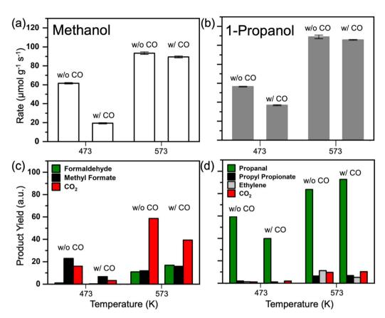
Fig. 3 The rate of (a) methanol and (b) 1-propanol oxidation in the absence (w/o CO) and presence (w/CO) of co-fed 2% CO at 473 K and 573 K over  $Pd_3Au_{97}$  RCT-SiO<sub>2</sub>, and the corresponding yield of products during (c) methanol and (d) 1-propanol oxidation. Reaction conditions: 4% 1-propanol, 10% O<sub>2</sub>, 0 or 2% CO, balanced in He; total flow rate = 50 mL min<sup>-1</sup>;  $m_{cat} = 10.0$  mg.
