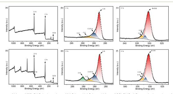
Fig. 4 XPS spectra of (a) acac(100)-PMO, in the regions of (b) C 1s and (c) O 1s; and (d) acac(100)-PMO@VO\_acac, in the regions of (e) C 1s and (f) O 1s.
