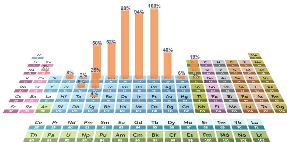
Fig. 2 Addition frequency of various elements of HEAs for HER and OER electrocatalysts from recent research. (The periodic table is from the Royal Society of Chemistry 107 ).
