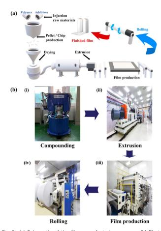
Fig. 2 (a) Schematic of the film manufacturing process. (b) Photographs of the required film-manufacturing machines. (i) Compounding polymers and additives. (ii) Film extrusion. (iii) Film production, and (iv) rolling of the film (final process). Courtesy of KM Corp.
