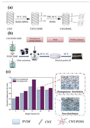
Fig. 14 (a) Schematic illustrating the preparation of CNT-POSS. (b) Schematic of the preparation of the CNT-POSS/PVDF composite membrane. (c) Thermal conductivity of CNT-COOH/PVDF and CNT-POSS/PVDF composite membranes with different filler loadings. Reproduced from ref. 121 with permission from Elsevier, copyright 2018.
