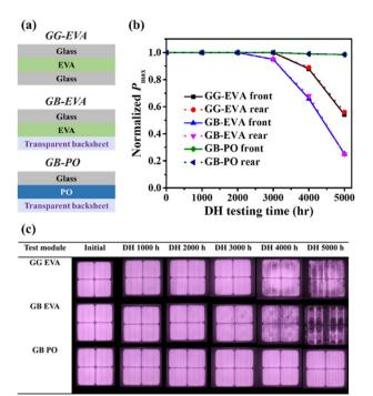
Fig. 16 (a) Schematic cross-section, (b) normalized  $P_{\rm max}$  retention, and (c) EL images of PV modules with different configurations (GG EVA, GB EVA, GB PO). Reproduced from ref. 134 with permission from IOP science, copyright 2018.
