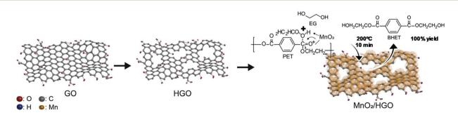
Scheme 18 Glycolysis of PET with EG (200  $^{\circ}$ C, 10 min) in the presence of MnO<sub>2</sub>/HGO as the catalyst. Reproduced with permission of ref. 88a. Copyright (2021) Elsevier.
