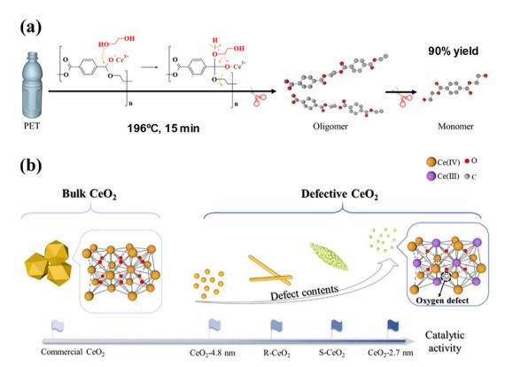
Scheme 15 (a) PET glycolysis (196 °C, 15 min) procedure over defective  $CeO_2$  NPs. (b) Structures and catalytic activities of  $CeO_2$  NPs with different morphologies. Reproduced with permission of ref. 56. Copyright (2022) American Chemical Society.
