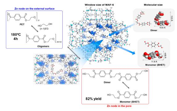
Scheme 20 Proposed mechanism for PU degradation at MAF-6 (180 °C, 4 h), together with size of both MAF-6 and, dimer and monomer (BHET). Adapted with permission of ref. 61. Copyright (2021) ACS.
