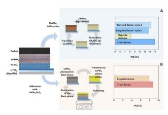
Fig. 6 Remanufacturing methodologies for triple-mesoscopic carbon-PSCs device architectures applying: (A) a methylamine gas restoration treatment (Reproduced with permission from ref. 46. Copyright 2017, John Wiley and Sons Inc.) and (B) restoration of allinorganic CsPbI<sub>3</sub> perovskite through thermal treatment (Adapted from ref. 80, available under a Creative Commons CC BY licence).
