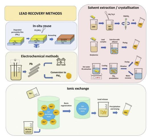
Fig. 3 Schematic of Pbl<sub>2</sub> recovery through different methods: in situ reuse, electrochemical methods, solvent extraction and crystallisation, and adsorption and ionic exchange.
