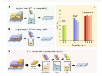
Fig. 1 Schematic of single-solvent TCO-substrate recovery method using (A) an alkaline solution or (B) dimethilformamide. (C) Multisolvent TCO recovery methods. (D) Performance of the devices fabricated with recycled TCO substrates as reported by Augustine et al., <sup>17</sup> Huang et al. <sup>18</sup> and Binek et al. <sup>15</sup>
