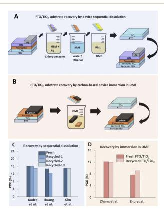
Fig. 2 (A) Sequential dissolution of perovskite device components by a multi-step, multi-solvent method. (B) Single-solvent method for the recovery and reuse of TCO/TiO<sub>2</sub> substrates. Efficiencies reported for (C) sequential dissolution<sup>22,23,26</sup> and (D) single-solvent recovery of TCO/TiO<sub>2</sub>.<sup>24,25</sup>
