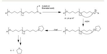
Fig. 8 Proposed mechanism for the ring-closing depolymerization of PTHF with acidic catalysts.<sup>54</sup>
