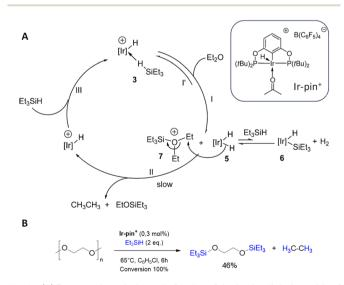
**Fig. 6** (A) Proposed catalytic cycle for the of the hydrosilylation with of diethylether with the iridium pincer complex Ir-pin<sup>+</sup>. (adapted with permission from The America Chemical Society, ©2008).<sup>48</sup> (B) Reaction conditions for the iridium-catalyzed depolymerization of PEG.<sup>49</sup>
