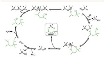
Fig. 20 Postulated reaction mechanism for the base-catalyzed depolymerization of PDMS with hexylene glycol. Reprinted with permission from The American Chemical Society, © 2023.<sup>146</sup>
