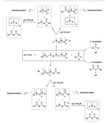
Fig. 24 Proposed mechanism for the depolymerization of PDMS catalysed by iron salts. Reprinted with permission of Wiley, © 2014.<sup>170</sup>
