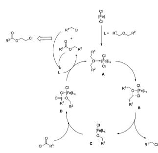
Fig. 2 Proposed catalytic cycle for the iron-catalysed depolymerisation of polyethers to chloroesters (reprinted with permission from Wiley, @2012).<sup>13</sup>
