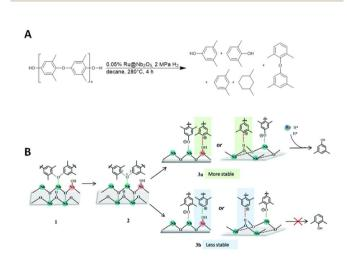
Fig. 12 (A) of PPO via hydrogenolysis in the presence of a supported ruthenium catalyst ( $Ru@Nb_2O_5$ ). (B) Proposed reaction mechanism (adapted with permission from The Royal society of Chemistry, ©2021).<sup>38</sup>
