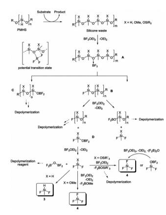
Fig. 22 Proposed mechanism for the depolymerization of silicones catalyzed by boron trifluoride. Reprinted with permission of Springer Nature, © 2015.<sup>165</sup>
