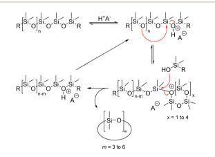
Fig. 14 Reaction mechanism for acid-catalysed depolymerisation of siloxanes.
