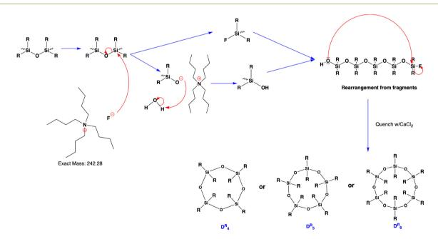
Fig. 23 Reaction mechanism for the depolymerization of PDMS catalysed by tetrabutylammonium fluoride. (Reprinted with permission of the American Chemical society, © 2021).<sup>167</sup>
