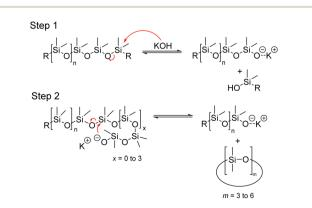
Fig. 15 General mechanism of base-catalysed depolymerization of polysiloxanes.
