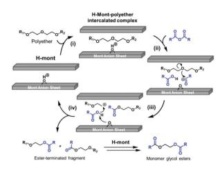
Fig. 5 Proposed catalytic cycle for the H-mont-catalysed depolymerisation of polyethers to glycol diesters (reprinted with permission from The Royal society of Chemistry, ©2017).<sup>34</sup>
