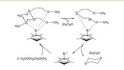
Fig. 9 Proposed reaction mechanism for the production of dioxane from dimethyl ether, catalysed by Cp\*Si<sup>+</sup>. (reprinted with permission from Wiley, ©2011).<sup>55</sup>
