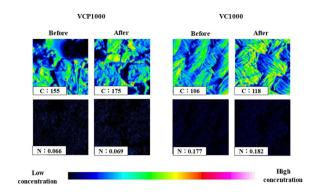
Fig. 8 The qualitative analysis of the adsorbent surfaces before and after adsorption.
