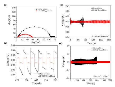
Fig. 3 Electrochemical testing of Li symmetrical cells. (a) Nyquist plots obtained from the EIS test, galvanostatic plating/stripping cycle test, (b) current density of  $0.5 \, \text{mA cm}^{-2}$  and capacity of  $1 \, \text{mA} \, \text{h cm}^{-2}$ , (c) test profile between 675 to 695 cycling hours, and (d) current density  $2 \, \text{mA cm}^{-2}$  and capacity of  $1 \, \text{mA} \, \text{h cm}^{-2}$ .
