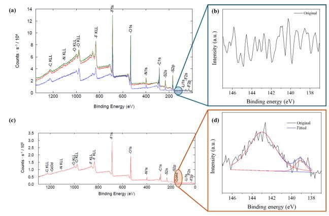
Fig. 2 XPS spectra for post-cycling LMA surfaces without (a and b) and with (c and d) Gd(NO<sub>3</sub>)<sub>3</sub> electrolyte additive. Multiple scans are shown in (a).
