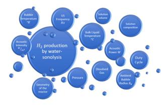
Fig. 2 Factors affecting hydrogen production by water-sonolysis
