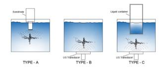
Fig. 4 Common configuration of a sonoreactor
