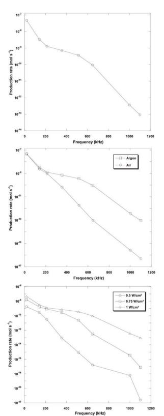
Fig. 6 Hydrogen production as a function of frequency, atmosphere and intensity. $^{70}$
