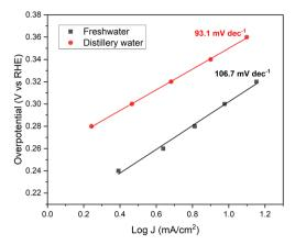
Fig. 4 Tafel plots of Ni<sub>2</sub>Se<sub>3</sub> in freshwater and distillery wastewater electrolytes.
