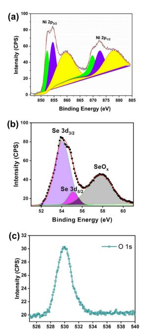
Fig. 2 (a) High resolution of Ni 2p, (b) Se 3d, and (c) O 1s spectra of XPS using the as-synthesized Ni<sub>2</sub>Se<sub>3</sub> powder sample.
