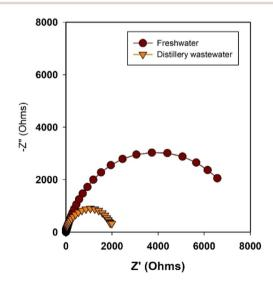
Fig. 5 Nyquist plots of Ni<sub>2</sub>Se<sub>3</sub> (anode) and Ni mesh (cathode) in both freshwater and distillery wastewater electrolytes. It is important to note that impedance measurements were conducted at open circuit potential.
