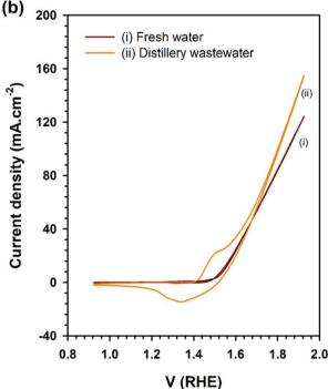
Fig. 3 (a) Linear sweep voltammogram results of stainless steel and Ni<sub>2</sub>Se<sub>3</sub> nanoparticles coated stainless steel substates in freshwater and distillery wastewater electrolyte. (b) CV of Ni<sub>2</sub>Se<sub>3</sub>/SS anode in freshwater and distillery wastewater-based electrolyte. Note that the concentration of the electrolyte was 1 M NaOH.
