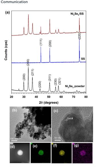
Fig. 1 (a) XRD pattern of Ni<sub>2</sub>Se<sub>3</sub> powder, stainless steel substrate (SS) and Ni<sub>2</sub>Se<sub>3</sub> coated SS (Ni<sub>2</sub>Se<sub>3</sub>/SS). HRTEM images of Ni<sub>2</sub>Se<sub>3</sub> powder (b) at 100 nm scale and (c) 10 nm scale. (d) Elemental mapping of Ni<sub>2</sub>Se<sub>3</sub> uniformly dispersing the elements of (e) Ni, (f) Se and (g) O.
