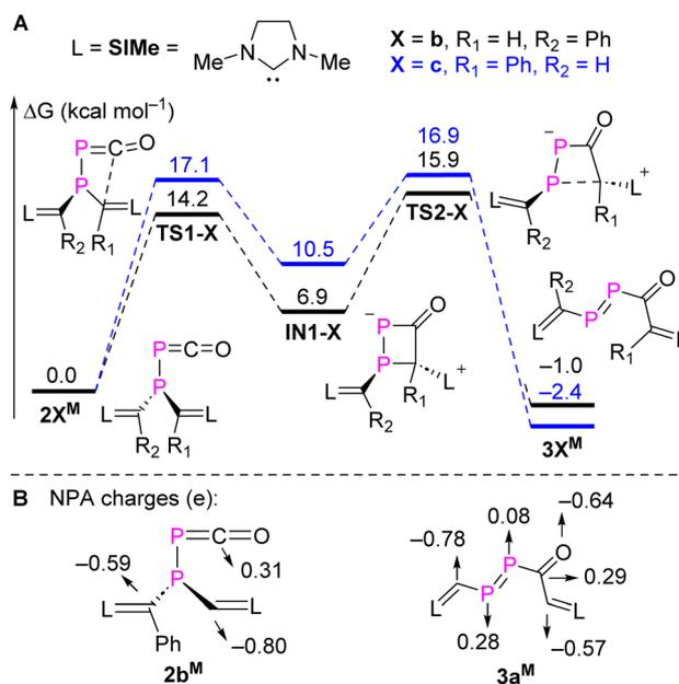
Fig. 3 (A) MERPs of the selective intramolecular rearrangement of **2b<sup>M</sup>**, and (B) selected NPA charges of **2b<sup>M</sup>** and **3a<sup>M</sup>** at M062X/Def2TZVP-SMD(toluene)//M062X/Def2SVP level of theory.
