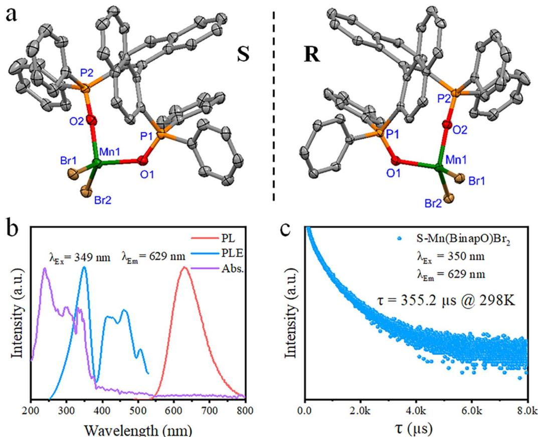
Fig. 1 (a) Visualization of the single crystal structures of the complexes *S*-Mn(Binapo)Br<sub>2</sub> (left) and *R*-Mn(Binapo)Br<sub>2</sub> (right). (b) Room temperature excitation and emission spectra and UV absorption spectra of *S*-Mn(Binapo)Br<sub>2</sub>. (c) PL decay lifetime curve of *S*-Mn(Binapo)Br<sub>2</sub>.
