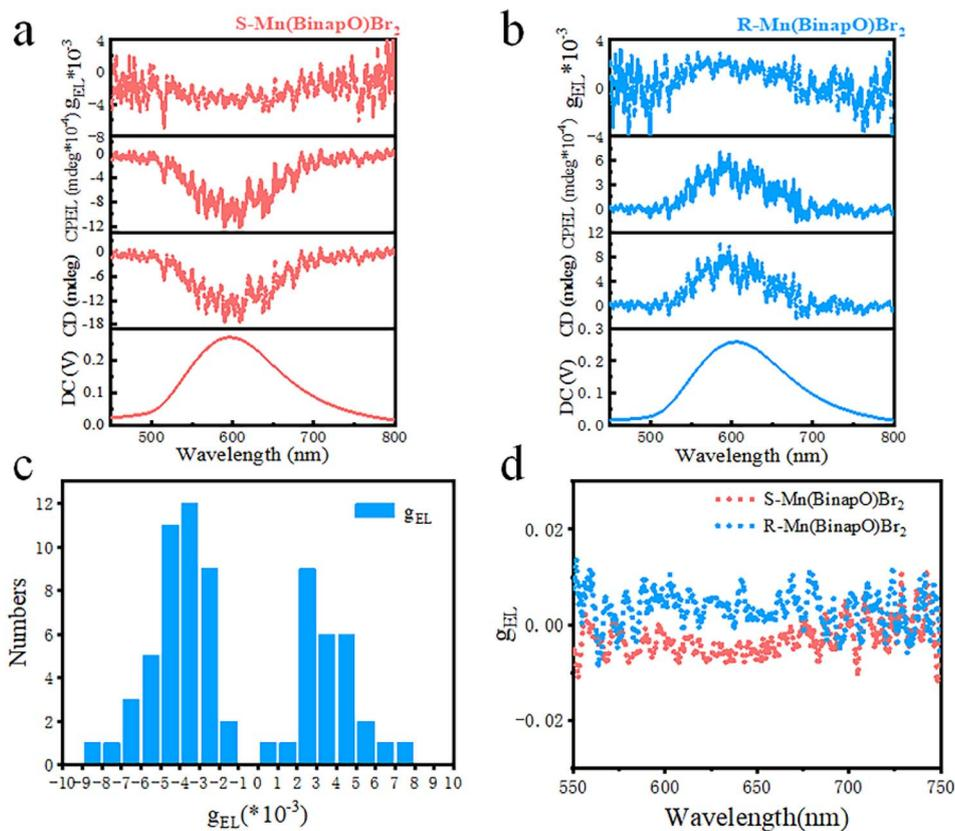
Fig. 4 Circularly polarized electroluminescence (CPEL) spectra of *S*-Mn(Binapo)Br<sub>2</sub> (a) and *R*-Mn(Binapo)Br<sub>2</sub> (b) with DC, CD, CPEL emission and  $g_{EL}$ . (c) Statistical plot of the CPEL asymmetry factor for doped OLED devices. (d) Maximum CPEL asymmetry factor curve for (*R/S*)-Mn(Binapo)Br<sub>2</sub>.
