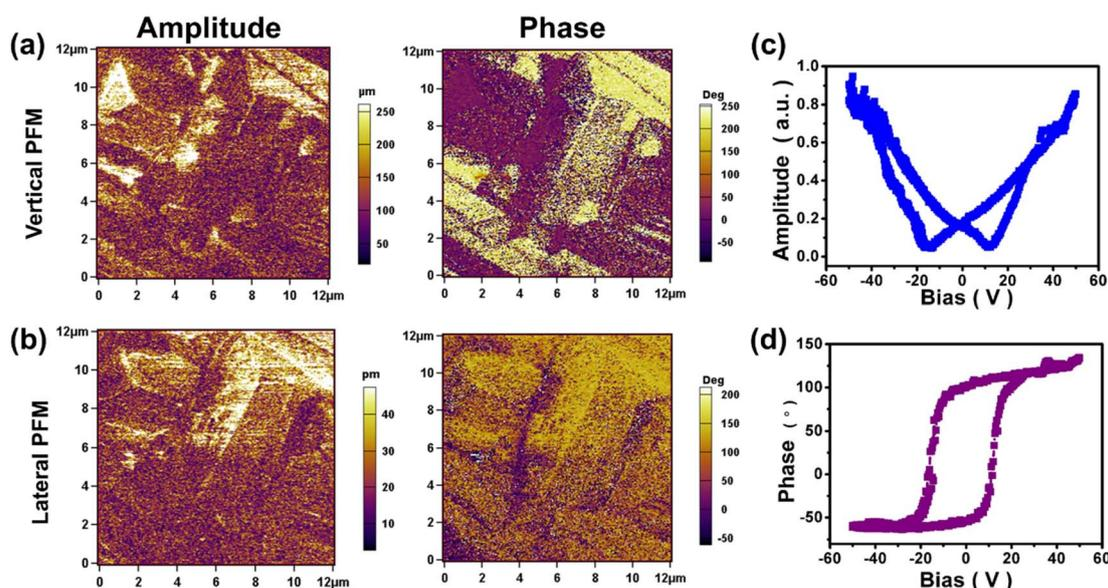
Fig. 3 Domain structure of **1**. Vertical (a) and lateral (b) PFM amplitude and phase images for a polycrystalline film of **1**; vertical PFM amplitude (c) and phase (d) signals as functions of the tip voltage for a selected point.
