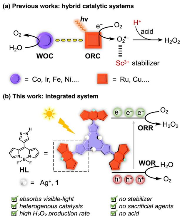
Scheme 1 Schematic illustration of (a) conventional metal-based hybrid catalytic systems and (b) a Ag-CTC complex in this work for photosynthesis of  $\text{H}_2\text{O}_2$ . (ORC and WOC mean the oxygen reduction catalyst and water oxidation catalyst).
