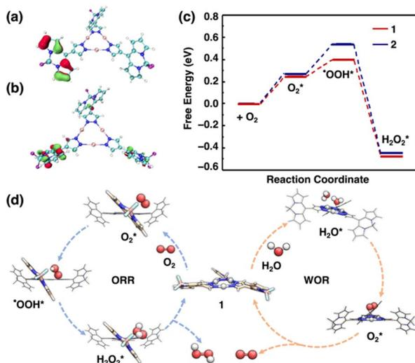
Fig. 5 (a) HOMO and (b) LUMO of **1** in the optimized structure (iso-value = 0.05 a.u.). (c) Calculated free energy for  $H_2O_2$  formation from  $O_2$  at the DFT-D3 (BJ) level of theory. (d) The proposed photocatalytic mechanism for  $H_2O_2$  synthesis in the presence of photocatalyst **1** (\* denoted as surface-adsorbed).
