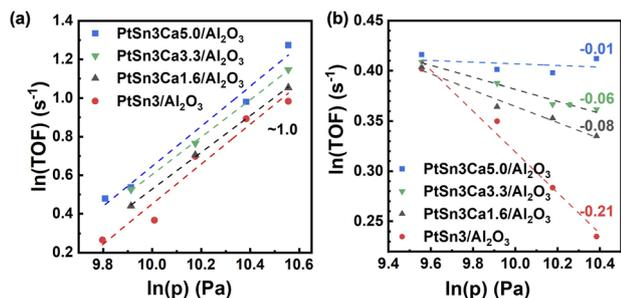
Fig. 4 TOF of propane as a function of (a) propane partial pressure and (b) hydrogen partial pressure on PtSn3/Al<sub>2</sub>O<sub>3</sub> catalysts with different Ca contents; catalytic conditions: atmospheric pressure, 873 K, and 5 mg of catalysts.
