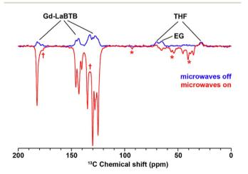
Fig. 8 <sup>13</sup>C MAS NMR spectra acquired for 23.5 mM Gd-LaBTB loaded with EG/THF at 100 K with (red) or without (blue) microwaves at the optimal field position (negative lobe in the <sup>13</sup>C field-sweep profile shown in Fig. 5). Asterisks indicate spinning side bands. Daggers indicate new MOF resonances appearing upon introduction of EG/THF.
