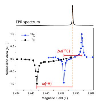
Fig. 5 DNP field-sweep profiles acquired for <sup>13</sup>C (blue) and <sup>1</sup>H (black) nuclei in Gd-LaBTB sample with the target Gd(III) concentration of 6 mM. The sample was stabilized until a constant  $T_1(^1H)$  was measured without "freeze-thaw" cycles. Spectra were recorded with polarization times of 40 and 4.5 s for <sup>13</sup>C and <sup>1</sup>H, respectively. At the top, the simulated EPR spectrum of Gd-LaBTB at 9.4 T and electron frequency of 263.5 GHz is shown.
