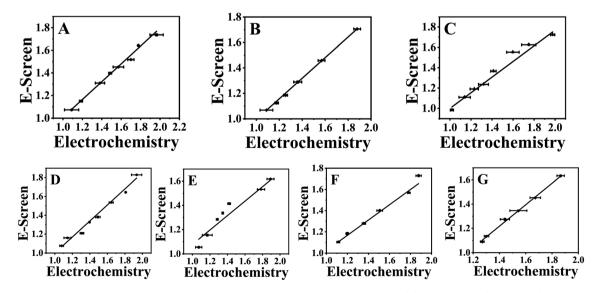
Fig. 4 Correlation fitting diagram between electrochemical method and E-Screen method. (A)  $GA_3$  (B) ETH, (C) NAA, (D)  $GA_3$ : ETH = 1:1, (E)  $GA_3$ : NAA = 1:1, (F) ETH: NAA = 1:1, (G)  $GA_3$ : ETH: NAA = 1:1.
