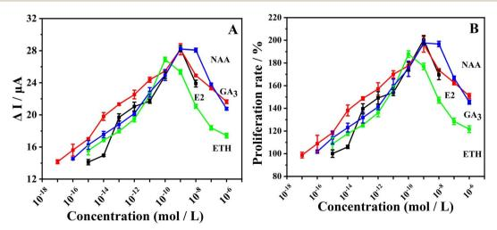
Fig. 2 Electrochemical signal and proliferation rate of estrogen-free MCF-7 cells exposed to PGRs were detected by electrochemical method. (A) change in electrochemical signal, (B) change in cell proliferation rate. Working electrode: MWCNTs/GCE, enrichment time: 360 s, applied potential: 0 V. Cell concentration:  $1 \times 10^6$  cells per dish, drug action time: 72 h. Control group: E2.
