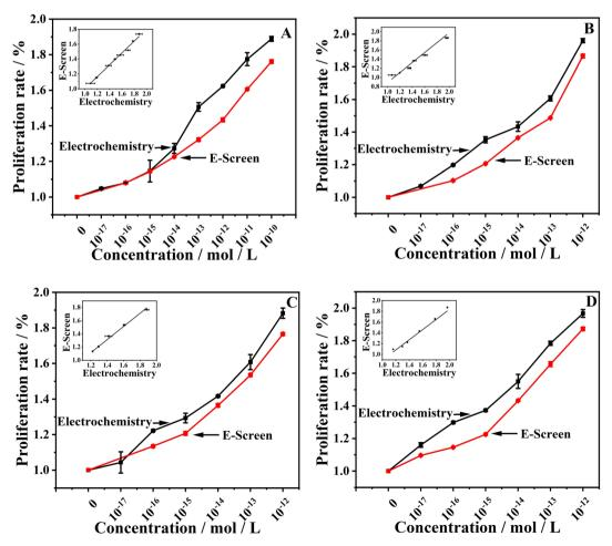
Fig. 5 The electrochemical and E-Screen methods detect the cell proliferation rate of PGRs at environmentally relevant concentrations. (A)  $GA_3$ : ETH = 1:5, (B)  $GA_3$ : NAA = 4:1, (C) ETH: NAA = 20:1, (D)  $GA_3$ : ETH: NAA = 4:20:1. Inset: correlation fitting between electrochemical method and E-Screen method.
