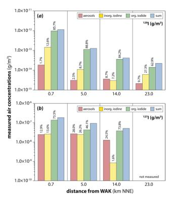
Fig. 9 Air concentrations of (a) <sup>129</sup>I and (b) <sup>127</sup>I in various chemical forms at four sampling locations NNE from WAK in the dominant downwind direction, as measured between June and September 1987. This figure was modified with permission from Wershofen and Aumann. <sup>105</sup> Copyright 1989 Elsevier.
