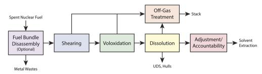
Fig. 2 Block flow diagram for aqueous head-end processing. 10 This figure was reprinted with permission. Copyright 2008 CRESP.
