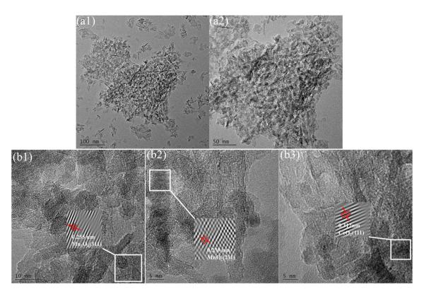
Fig. 1 TEM images (a1 and a2) and HRTEM images (b1-b3) of Ce-Mn/γ-Al<sub>2</sub>O<sub>3</sub>.
