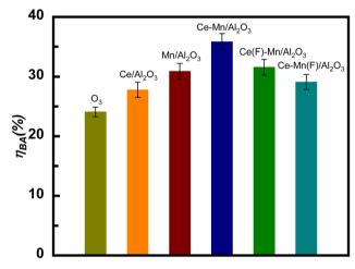
Fig. 7 Comparison of benzoic acid degradation efficiency between single and catalytic ozonation by Ce–Mn/Al<sub>2</sub>O<sub>3</sub>, Ce–Mn(F)/Al<sub>2</sub>O<sub>3</sub> and Ce(F)–Mn/Al<sub>2</sub>O<sub>3</sub> (V=1000 mL,  $c_{\rm BA}=50$  mg L<sup>-1</sup>,  $m_{\rm S}=0.5$  g L<sup>-1</sup>,  $C_{\rm O3}=7.5$  mg L<sup>-1</sup>, time = 15 min).
