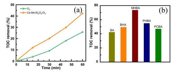
Fig. 9 TOC removal of benzoic acid solution in the single ozonation and catalytic ozonation (a) and TOC removal of benzoic acid derivatives during the catalytic ozonation (b) (V = 1000 mL,  $c_0 = 50 \text{ mg L}^{-1}$ ,  $m_s = 0.5 \text{ g L}^{-1}$ ,  $C_{O_s} = 7.5 \text{ mg L}^{-1}$ , time = 60 min).
