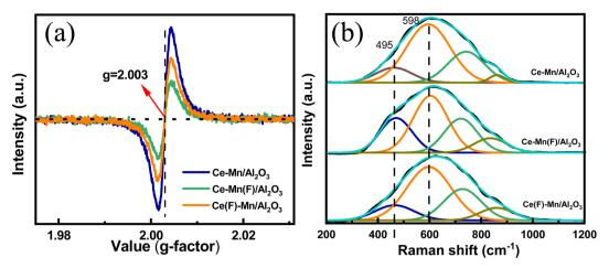
Fig. 6 EPR (a) and Raman (b) spectra of Ce-Mn/Al<sub>2</sub>O<sub>3</sub>, Ce-Mn(F)/Al<sub>2</sub>O<sub>3</sub> and Ce(F)-Mn/Al<sub>2</sub>O<sub>3</sub>.
