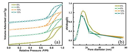
Fig. 3  $N_2$  adsorption and desorption isotherms (a) and pore size distribution curves (b) of Ce-Mn/Al<sub>2</sub>O<sub>3</sub> with different metal loadings.
