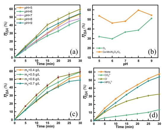
Fig. 8 Effect of pH (a) and (b), catalyst dosage (c) and anions (d) on the catalytic ozonation degradation efficiency of benzoic acid
