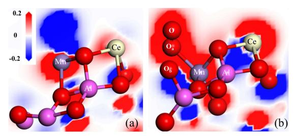
Fig. 12 The differential charge density adjacent to the oxygen vacancy of  $Ce-Mn/Al_2O_3(110)$  surface before (a) and after (b) ozone adsorption.
