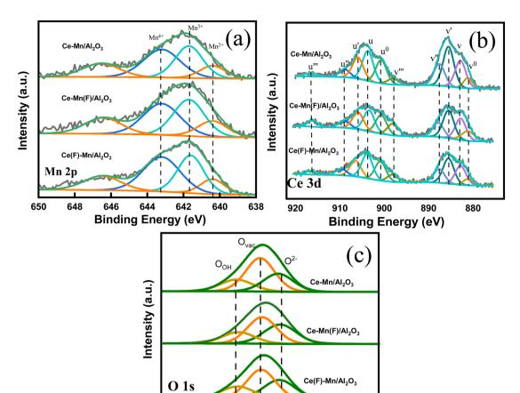
Fig. 5 High resolution Mn 2p (a), Ce 3d (b) and O 1s (c) XPS spectra of Ce-Mn/Al<sub>2</sub>O<sub>3</sub>, Ce-Mn(F)/Al<sub>2</sub>O<sub>3</sub> and Ce(F)-Mn/Al<sub>2</sub>O<sub>5</sub>.
