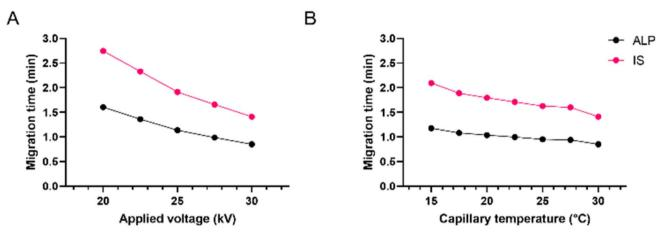
Effect of (A) applied voltage and (B) capillary temperature on ALP and IS migration times; 25 mM borate at pH 9.3.
