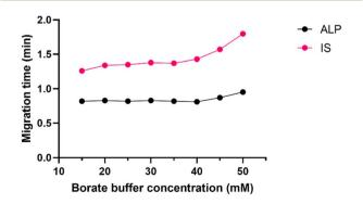
Fig. 3 Effect of borate buffer concentration (15–50 mM) on ALP and IS migration times, pH 9.3, 30  $^{\circ}$ C, 30 kV.
