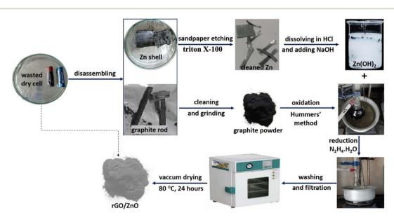
Scheme 1 Synthesis of rGO/ZnO utilizing graphite and Zn collected from wasted dry cells
