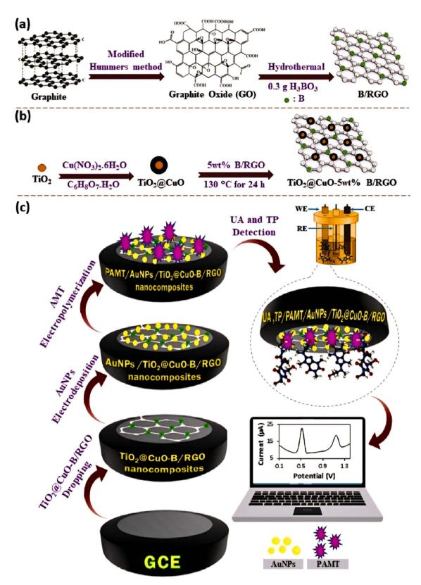
Fig. 3 Procedure for the preparation of (a) B/RGO nano-sheet, (b) TiO<sub>2</sub>@CuO-B/RGO nanocomposites, and (c) design of electrochemical sensor for the simultaneous detection of UA and TP by the PAMT/AuNPs/TiO<sub>2</sub>@CuO-B/RGO nanocomposite. Reprinted with permission from ref. 117. Copyright (2023), Elsevier.
