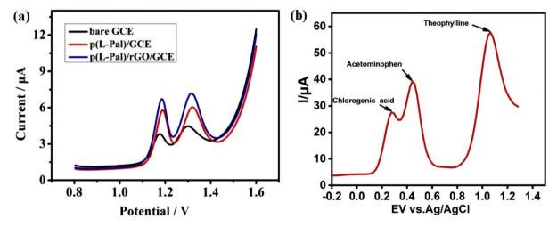
Fig. 4 (a) DPV of 40 μM TP on different electrodes in 10 mM H<sub>2</sub>SO<sub>4</sub>. Reprinted with permission from ref. 126. Copyright (2021), Elsevier and (b) DPV of 0.1 M TP current response on ZnONPs-MWCNTs-Cyt c-GCE electrode with the addition of various interfering species. Reprinted with permission from ref. 131. Copyright (2020), Elsevier.
