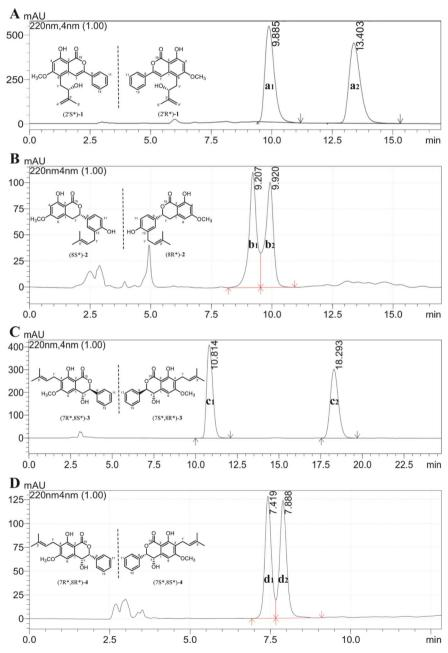
Fig. 4 Chiral analysis of compounds 1-4. (A) Relative peak area ratio of compound 1 was calculated as a1: a2 = 49.4: 50.6; (B) relative peak area ratio of compound 2 was calculated as b1: b2 = 51.3: 48.7; (C) relative peak area ratio of compound 3 was calculated as c1: c2 = 49.2: 50.8; (D) relative peak area ratio of compound 4 was calculated as d1: d2 = 50.5: 49.5.
