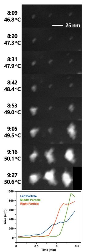
Fig. 7 Selected STEM images from Movie 2† showing BiOCl formation and growth from BiClLac. Images are spaced ca. 11 s apart with times and temperatures indicated. The black area in the last frame is where the particle clusters drifted near the edge of the field of view and was applied during drift correction. Scale bar applies to all images. Below the images is a plot of the clusters' 2D area over time. Image processing steps for Movie 2 are shown in Movie S1.†
