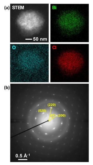
**Fig. 6** (a) STEM image and EDS mapping of a synthesized BiOCl particle, with bismuth in green, oxygen in blue, and chlorine in red. The oxygen signal is high outside of the particle due the oxygen in water. Scale bar applies for all four images. STEM image field of view is 289 nm  $\times$  289 nm (802  $\times$  802 pixels) with an EDS signal binning factor of 2. (b) SAED pattern of particle in (a) with reflections indexed.
