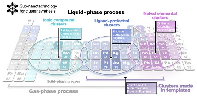
Fig. 2 A rough sketch of a map for the classification of suitable methods for atomic cluster synthesis depending on the chemical element composition.
