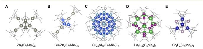
Fig. 4 Crystal structures of (A)  $Zn_9(C_5Me_5)_6$ .<sup>87</sup> (B)  $Cu_3Zn_4(C_5Me_5)_5$ ,<sup>89</sup> (C)  $Cu_{43}Al_{12}(C_5Me_5)_{12}$ ,<sup>90</sup> (D)  $La_9l_{18}(C_5Me_5)_9$ ,<sup>91</sup> and (E)  $Cr_4P_4(C_5Me_5)_4$ .<sup>93</sup> Zn: gray, Cu: blue, Al: light blue, La: green, I: violet, Cr: dark blue, P: grayish pink, and C: grayish bone. Figures are reproduced from (A) CCDC 1434844, (B) CCDC 1854852, (C) CCDC 1845365, (D) CCDC 1992039, and (E) CCDC 984791.
