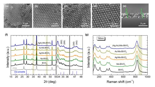
Fig. 2 Plan view SEM images for (a) PC239, (b) PC287, (c) PC340, (d) PC418, and cross section for (e) PC340 inverse opal films. (f) XRD patterns and (g) Raman spectra of Ag,Au-modified Mo-BiVO<sub>4</sub> PC340 films compared to the pristine Mo-doped and undoped BiVO<sub>4</sub>. The XRD patterns of the FTO substrate and the ms phase (JCPDS 014-0688) are also displayed, while the right panels in (f) depict in detail the shaded areas of the XRD patterns.
