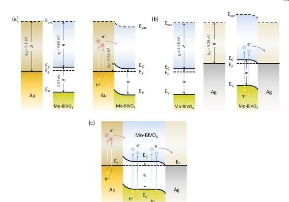
Fig. 8 Schematic of the dominant charge transfer routes for (a) Au/Mo-BiVO<sub>4</sub>, (b) Ag/Mo-BiVO<sub>4</sub> and (c) (Ag,Au)/Mo-BiVO<sub>4</sub>.
