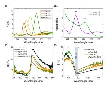
Fig. 5 (a) Specular reflectance (R%) at 15° incidence (R%) for the Mo-BiVO<sub>4</sub> PC films and (b) LSPR absorbance of Ag and Au NP suspensions (c) diffuse reflectance (DR%) and the corresponding (d) Kubelka-Munk transforms F(DR) for the Aq, Au-modified PC340 films.
