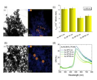
Fig. 9 TEM images and the corresponding V and Au EDX elemental maps for Mo-BiVO $_4$  PC340 films surface modified by Au NPs of (a) 50 and (b) 80 nm diameters. (c) Size dependent TC degradation rates at +1.0 V vs. Ag/AgCl under visible light and (d) DR (%) spectra for the Au/Mo-BiVO $_4$  PC340 photoelectrodes with Au NPs of different diameters.
