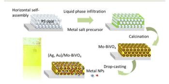
Fig. 1 Schematic illustration of the fabrication of (Ag,Au)/Mo-BiVO<sub>4</sub> inverse opal films.
