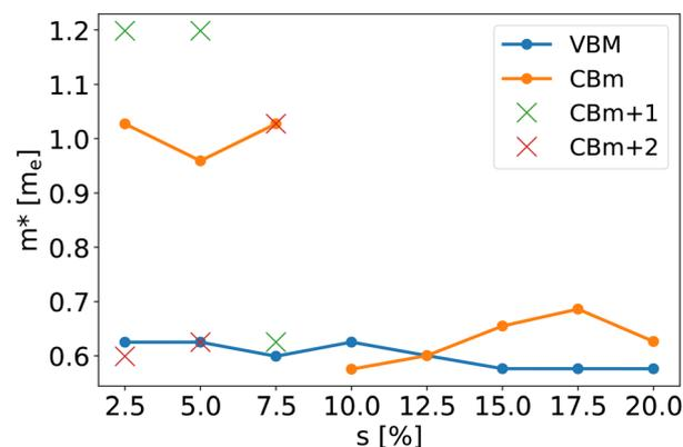
Fig. 6 Effective masses of the highest valence band (VBM) and the lowest unoccupied states (CBM) at the  $\Gamma$  point.
