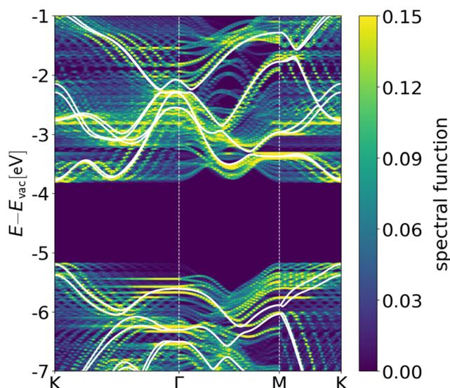
**Fig. 3** Unfolded band structure of the nanowrinkle with  $s = 10\%$  represented by the spectral function. The white lines indicate the band structure of the flat and unstrained MoSe<sub>2</sub> monolayer. The energy scale is offset with respect to the vacuum level ( $E_{\text{vac}}$ ) set to zero.
