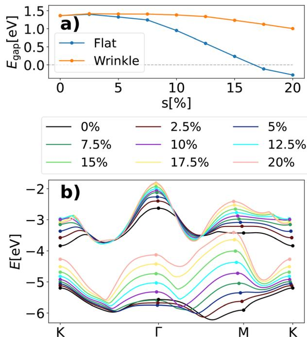
**Fig. 4** (a) Band gap ( $E_{\text{gap}}$ ) vs. strain ( $s$ ) of the considered MoSe<sub>2</sub> nanowrinkles (orange) and of the flat monolayers under the same amount of uniaxial strain in their hexagonal UC (blue). (b) Highest-occupied and lowest-unoccupied band of flat MoSe<sub>2</sub> under the displayed values of strain. The deformation of the BZ leads to different distances between the high-symmetry points in the K-path and hence they are shown separately for each strain value.
