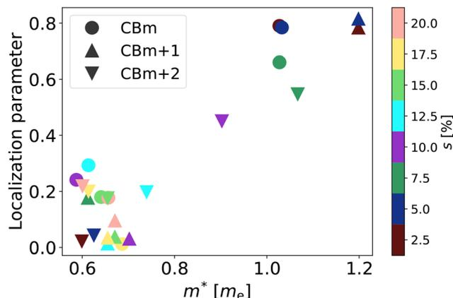
**Fig. 8** Localization parameter  $L$  mapped against the effective mass  $m^*$  for the 3 lowest states in the conduction band at  $\Gamma$ . States with  $m^* < 0.8m_e$  are densely clustered in the area with low  $L$ , while the ones with higher effective mass are more dispersed, but still clearly correspond to higher values of  $L$ .
