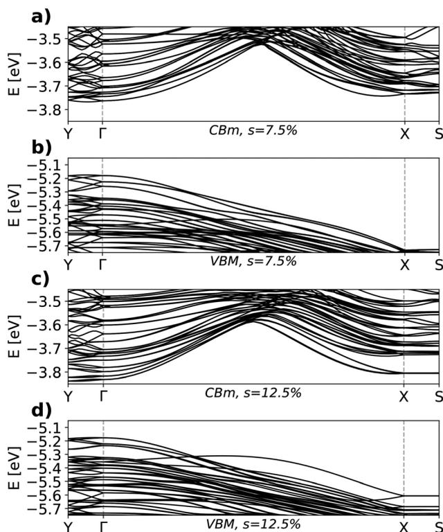
Fig. 5 Band structure in the orthorhombic BZ for the nanowrinkle with  $s = 7.5\%$  [conduction region in (a) and valence region in (b)] and  $s = 12.5\%$  [conduction region in (c) and valence region in (d)].
