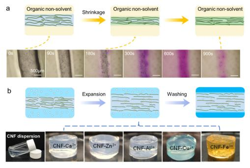
**Fig. 8** Schematic presentations of the coagulation process using different coagulation baths and the corresponding still-wet fibers: (a) organic non-solvents. Adapted with permission from ref. 51. Copyright 2023 Elsevier. (b) Ion solutions containing acids or salts. Adapted with permission from ref. 126. Copyright 2013 ACS.
