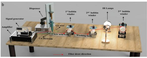
Fig. 11 The representative schematic diagrams of the integrated wet spinning device for the continuous fabrication of CNF wet-spun fibers with (a) in-built heaters<sup>61</sup> and (b) AC electric field.<sup>105</sup> Adapted with permission from ref. 61 and 105. Copyright 2022, 2023 Springer Nature.
