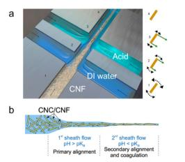
Fig. 6 (a) Schematic of a typical flow-focusing device with double channels used for CNF assembly.<sup>67</sup> (b) The schematic presentation of nanocellulose orientation and gelation in the microfluidic device.<sup>71</sup> Adapted with permission from ref. 71. Copyright 2019 Wiley.
