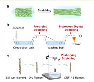
Fig. 9 Schematic presentation of (a) CNF network changes practically the CNF orientation during the wet stretching process, (b) pre-drying and in-process stretching processes and the (c) post-drying stretching process.<sup>51</sup> Adapted with permission from ref. 51. Copyright 2023
