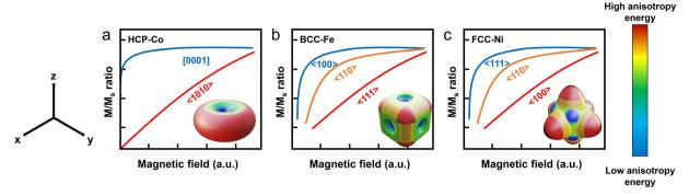
Fig. 3 Magnetocrystalline anisotropy of the simplest magnetic materials such as (a) hcp-Co, (b) bcc-Fe, and (c) fcc-Ni. The inset images in each figure represents magnetocrysalline ansisotropy energy. The red color represents high magnetic anisotropy energy resulting in a hard axis along that direction while the blue color represents low magnetic anisotropy energy forming an easy axis in the direction.
