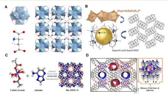
Fig. 3 (A) Structure of MIP-202(Zr). Reproduced with permission from ref. 59. (B) Structure of Cu10 cages. Reproduced with permission from ref. 60. Copyright 2021 American Chemical Society. (C) Structure of bio-MOF-11. Reproduced with permission from ref. 61. Copyright 2020 American Chemical Society. (D) Structure of SION-19. Reproduced with permission from ref. 62.
