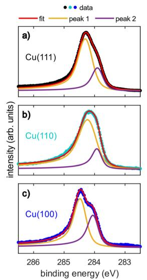
Fig. 2 (a-c) Soft X-ray photoelectron spectroscopy (SXPS) of azupyrene adsorbed on (a) Cu(111), (b) Cu(110), and (c) Cu(100). The data were acquired at a photon energy of 430 eV, the binding energy scale was corrected using a subsequent measurement of the Cu Fermi edge at the same photon energy. Nb. it was not possible to obtain a unique fit of the spectra, and these fits are presented here for illustrative purposes.
