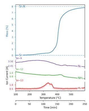
Fig. 6 Variations of mass (recorded by the TGA) and ion current (recorded by the mass spectrometer) as a function of time and temperature for the Sr-nitridation under 100% N<sub>2</sub>. Blue dashed lines: theoretical mass changes for no conversion (0%) and full conversion to Sr<sub>2</sub>N (7.99%) according to reaction (3). The ion current signals correspond to N2 (purple), NH3 (green), and H<sub>2</sub> (red).
