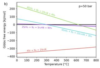
Fig. 3 Ellingham diagram of the nitridation step for reactions (3)–(6). Variation of the Gibbs free energy change per mol  $N_2$  as a function of temperature for (a) standard  $\Delta G_{\text{rxn}}^{\circ}$ ; and (b)  $\Delta G_{\text{rxn}}$  at 50 bar assuming 20% reaction extent.
