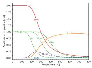
Fig. 5 Equilibrium composition of the Sr-H-N system as a function of temperature at 1 bar with initial conditions  $Sr_2N + 10H_2$ . Also shown are the NH<sub>3</sub> curves at 10 and 50 bar. Solid lines: solid phases; dashed lines: gaseous phases.
