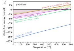
Fig. 4 Ellingham diagram of the hydrogenation step for the reactions (7)–(11). Variation of the Gibbs free energy change per mol  $H_2$  as a function of temperature for: (a) standard  $\Delta G_{\mathrm{rxn}}^{\circ}$ ; and (b)  $\Delta G_{\mathrm{rxn}}$  at 50 bar assuming 20% reaction extent.
