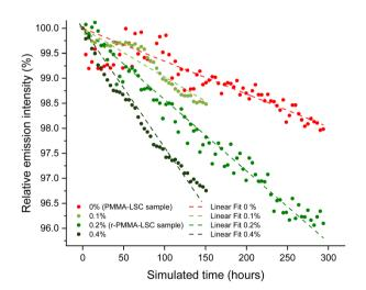
Fig. 4 Photodegradation studies with time under UV irradiation (1.14 Sun) at 70 °C for LSCs at increasing MIB concentrations. All samples contained 400 ppm LR305. PMMA LSC (with 0% MIB, red dashed line; Pearson's r = 0.86); PMMA LSC with added 0.1% MIB (light green dashed line: Pearson's r = 0.85); r-PMMA LSC (sample containing 0.2% MIB. green dashed line; Pearson's r = 0.86); PMMA LSC with added 0.4% MIB (dark green dashed line; Pearson's r = 0.84).
