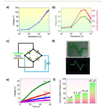
Fig. 5 (a) Voltage, (b) power and power density plots as a function of load resistance corresponding to the 5 wt% DIPAB/P(VDF-TrFE) fiberbased device. (c) Full-wave bridge rectifier circuit (schematic). Practical applications of the developed 5 wt% DIPAB/P(VDF-TrFE) fiber-based TENG device (d) towards glowing of LEDs, (e) charging of various capacitors and (f) their corresponding plots of accumulated charges.
