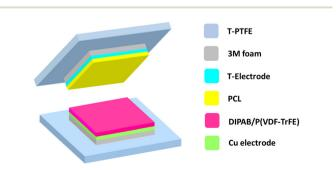
Fig. 1 Construction of the TENG device (schematic).
