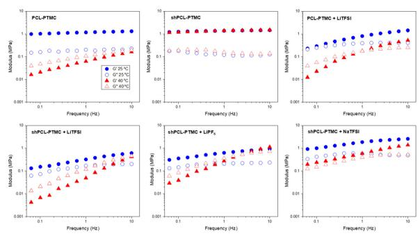
Fig. 1 Oscillatory sweep of HMW PCL-PTMC, shPCL-PTMC, and the polymer electrolytes containing LiTFSI, LiPF<sub>6</sub>, and NaTFSI at 25 °C and 40 °C
