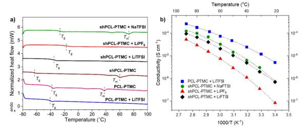
Fig. 2 (a) DSC analysis of shPCL-PTMC and self-healing polymer electrolytes; (b) Ionic conductivity of PCL-PTMC, shPCL-PTMC with LiTFSI, shPCL-PTMC with NaTFSI, and shPCL-PTMC with LiPF<sub>6</sub>. The dashed lines in (b) represent VFT fits.
