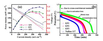
Fig. 7 Battery performance of SPES/E-PANI blend membranes. (a) Polarization curve and (b) open circuit potential of SPES/E-PANI blend membranes and Nafion 117
