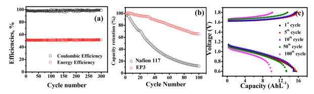
Fig. 6 Battery performance of E-PANI composite EP3 membranes. (a) Charge-discharge during 300 cycles at 140 mA cm<sup>-2</sup>. (b) Capacity retention with cycle number at 140 mA cm<sup>-2</sup>. (c) Capacity at different cycle numbers at 140 mA cm<sup>-2</sup>.
