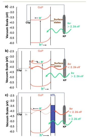
Fig. 7 Schematic band diagrams of GaP (a), In/GaP (b), and In/GaP/ HTL (c) layer stacks with charge separation based on surface photovoltage spectra. KP stands for Kelvin probe.
