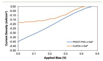
Fig. 9 Current-voltage curves for PEDOT:PSS-n-GaP device (blue) CuSCN-n-GaP device (orange) under simulated AM1.5G illumination.
