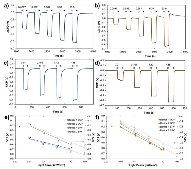
Fig. 8 Surface photovoltage (change in contact potential difference [ΔCPD]) and open circuit potential (OCP) measurements of PEDOT:PSS-n-GaP (a and c) and CuSCN-n-GaP (b and d) under variable light intensity (mW cm<sup>-2</sup>) from a 405 nm LED. White circles indicate when the LED is turned on and black circles indicate when the LED is turned off. Semi-logarithmic plot of OCP and surface photovoltage (SPV) vs. incident light power for PEDOT:PSS-n-GaP device (e) and CuSCN-n-GaP device (f).
