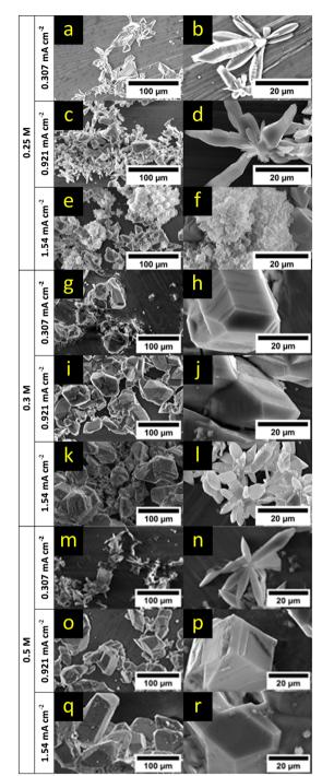
Fig. 4 SEM images after 8 h of magnesium deposition from a 0.25 M (a-f), 0.3 M (g-l) and 0.5 M (m-r) MeMgCl electrolyte solution. The applied current density (rows) can be derived from the subsection of each concentration.
