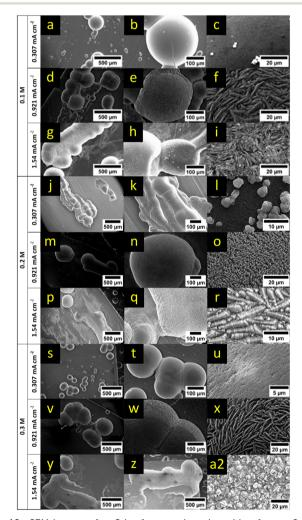
Fig. 10 SEM images after 8 h of magnesium deposition from a 0.1 M (a–i), 0.2 M (j–r) and 0.3 M (s–a2) Mg[B(hfip)<sub>4</sub>]<sub>2</sub> electrolyte solution. The applied current density (rows) can be derived from the subsection of each concentration.
