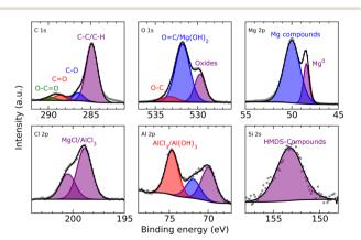
Fig. 8 C 1s (top left), O 1s (top middle), Mg 2p (top right) and Cl 2p (bottom left), Al 2p (bottom middle) and Si 2s (bottom right) XPS detail spectra of deposited Mg after 8 h from a 0.1 M Mg(HMDS)2-2AlCl3 solution with a current density of 1.54 mA cm<sup>-2</sup>.
