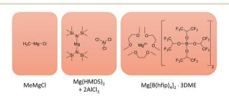
1 Structures of the MeMgCl, Mg(HMDS)<sub>2</sub>-2AlCl<sub>3</sub> and Mg[B(hfip)<sub>4</sub>]<sub>2</sub>·3DME electrolytes. In the case of Mg(HMDS)<sub>2</sub>-2AlCl<sub>3</sub> electrolyte, only the precursors are drawn, as a complex Schlenk equilibrium unfolds upon dissolving in a respective solvent. A detailed investigation of this behaviour was performed by Merrill and Schaefer. 18
