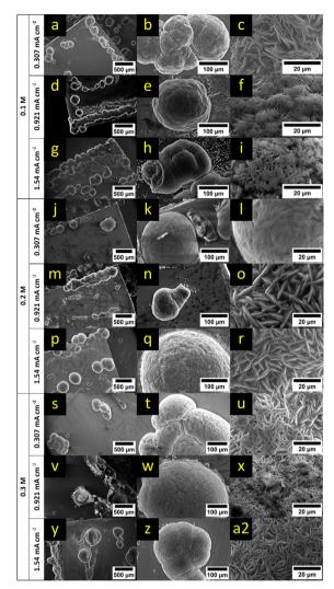
Fig. 7 SEM images after 8 h of magnesium deposition from a 0.1 M (a–i), 0.2 M (j–r) and 0.3 M (s–a2)  $Mg(HMDS)_2$ –2AlCl<sub>3</sub> electrolyte solution. The applied current density (rows) can be derived from the subsection of each concentration.
