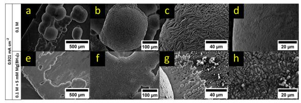
Fig. 13 SEM comparison of magnesium deposits from a 0.1 M Mg[B(hfip)<sub>4</sub>]<sub>2</sub> solution (a-d) and a Mg[B(hfip)<sub>4</sub>]<sub>2</sub> solution containing 5 mM Mg(BH<sub>4</sub>)<sub>2</sub> (e-h). The pictures (a)-(c) were already presented in Fig. 10d-f but were reused for better comparability with the additive. Pictures (c and d) show the surface of the largest and one of the smaller deposits featured in (b), respectively.
