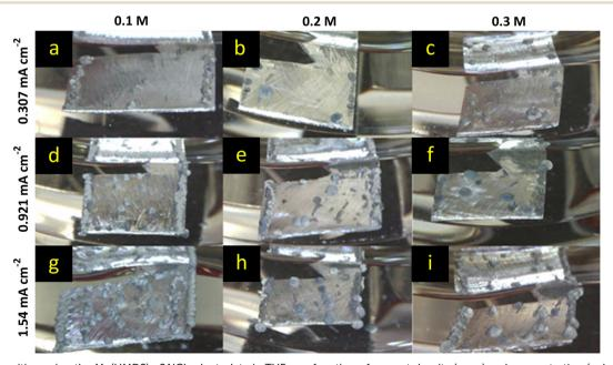
Fig. 6 Mg deposition using the Mg(HMDS)<sub>2</sub>–2AlCl<sub>3</sub> electrolyte in THF as a function of current density (rows) and concentration (columns) after 8 h of chronopotentiometry. The applied current density ranged from 0.307 mA cm<sup>-2</sup> (a-c) to 0.921 mA cm<sup>-2</sup> (d-f) and 1.54 mA cm<sup>-2</sup> (g-i) for electrolyte concentrations between 0.1 M and 0.3 M.
