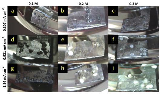
Fig. 9 Mg deposition using the Mg[B(hfip)<sub>4</sub>]<sub>2</sub> electrolyte in DME as a function of current density (rows) and concentration (columns) after 8 h of chronopotentiometry. The applied current density ranged from 0.307 mA cm<sup>-2</sup> (a-c) to 0.921 mA cm<sup>-2</sup> (d-f) and 1.54 mA cm<sup>-2</sup> (g-i) for electrolyte concentrations between 0.1 M and 0.3 M.
