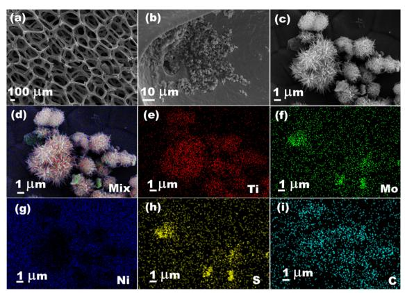
Fig. 6 (a-c) SEM images of the MQD@NFs drop-casted on the Ni foam before HER, elemental mapping for (d) mix (e) Ti, (f) Mo, (g) Ni, (h) S and (i) C.
