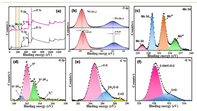
Fig. 5 XPS spectra of (a) full survey for MQD@NFs, (b) Ti and (c) Mo comparison before and after doping and (d) S, (e) C and (f) O for MQD@NFs.
