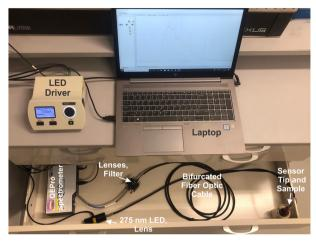
Fig. 2 Photograph of the portable fiber optic probe. The system is sufficiently compact to fit within a drawer or box and includes a bifurcated cable connecting the BioMOF-coated tip to both the UV LED excitation source and the ocean optics QEPro spectrometer.
