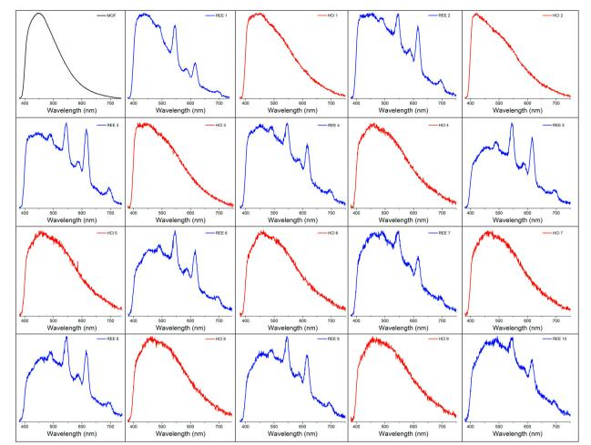
Fig. 4 Demonstration of qualitative reversible sensing of ~6 ppm terbium and europium across 10 sensing cycles; 0.3 M hydrochloric acid is used in between each measurement to restore the original emission signal of the BTC-1 MOF.
