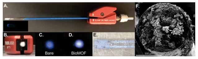
Fig. 1 Side view of a section of an optical fiber in a fiber optic terminator functionalized on one end by a BioMOF (A) (inset: MOF-coated tip with the 275 nm LED turned on), front view of the MOF-coated fiber optic tip (B), comparison of the fiber optic tip before (C) and after (D) MOF functionalization with the 275 nm LED turned on, optical microscope image of the MOF-functionalized fiber optic tip (E), and SEM image of the MOF-coated fiber optic tip (F).
